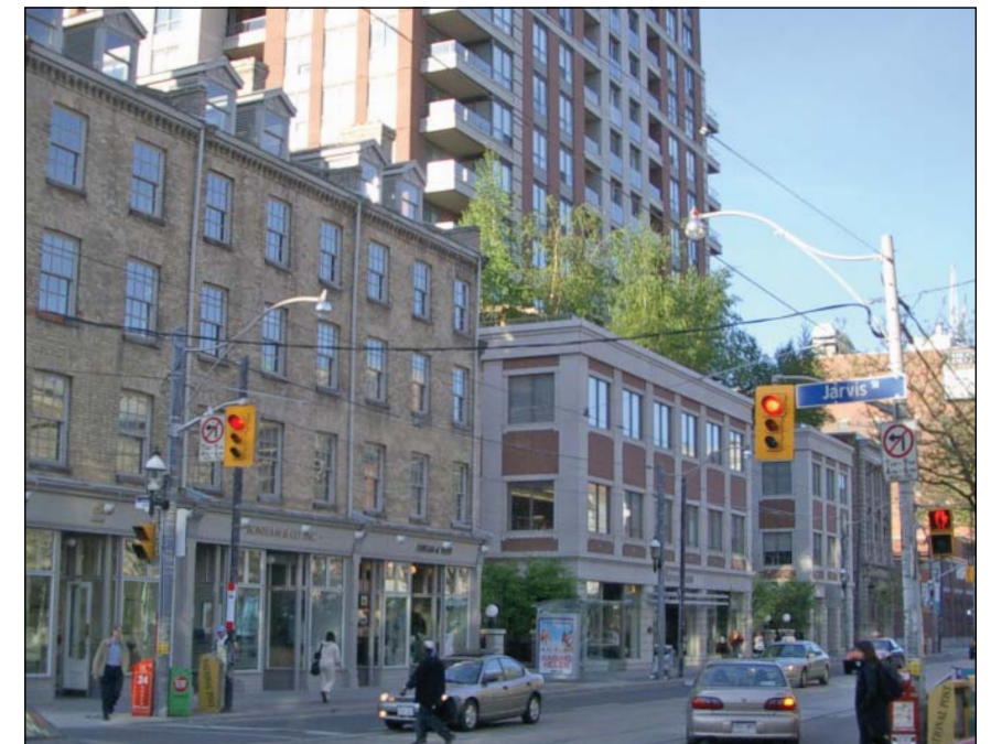
A new residential building in Toronto, Ontario uses a podium and generous setbacks to "fit in" with the surrounding street character.
